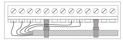
Figure C-10 Example of Cable Strain Relief
